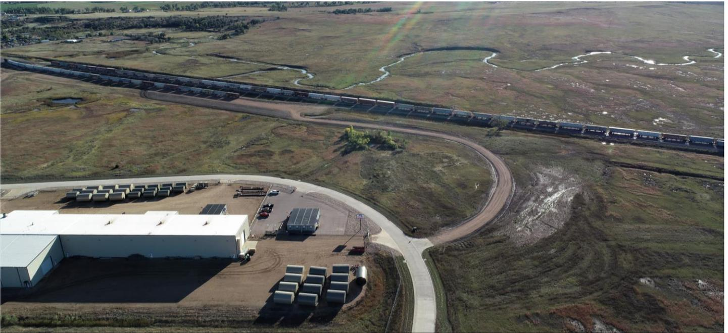
A new access road and additional siding space has been completed to serve a new rail customer for the Belle Fourche Industrial & Rail Park. The additional siding space accommodates off-loading equipment and the new access road allows for trucks to have easier access to the siding - creating a west entrance (across from Permian Tank) and an exit on the east side.
